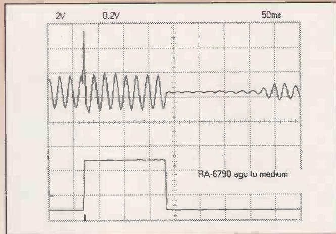
Fig. 2: The RA6790's audio response to a step r.f. input for 'medium' a.g.c. settings.
