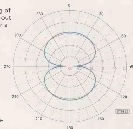
Fig. 2: Figure-8 dipole horizontal pattern.
