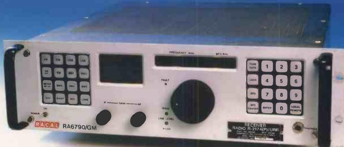
weighted for the right 'feel' and placed at just the right height above the bench top for comfortable operation. Above the tuning knob is a long l.c.d. which shows the operating frequency down to 1Hz, with a sub display showing b.f.o. offset to  $\pm 8\text{kHz}$  in steps of 10Hz. The b.f.o. display is only shown when in c.w. mode.
