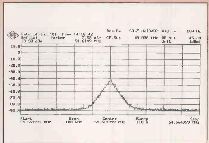
Fig. 4: The RA6790's first conversion oscillator plot, not as good as a RA1792!
