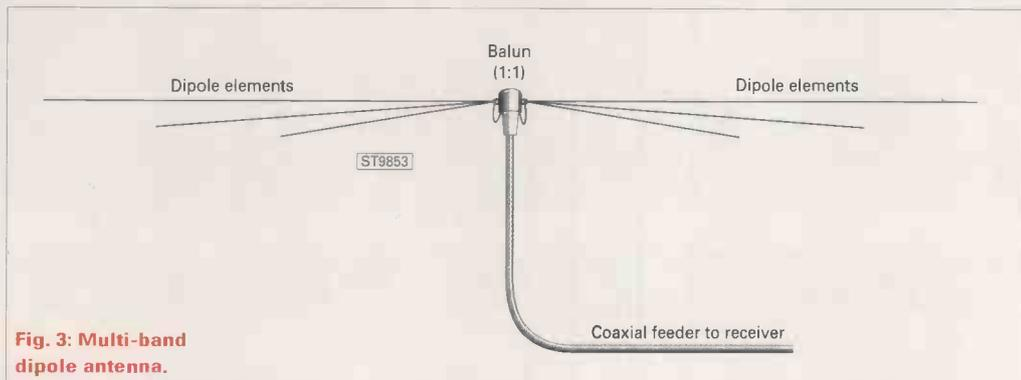
**Fig. 3: Multi-band dipole antenna.**
