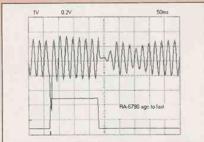
Fig. 1: The RA6790's audio response to a step r.f. input for 'fast' a.g.c. setting.
