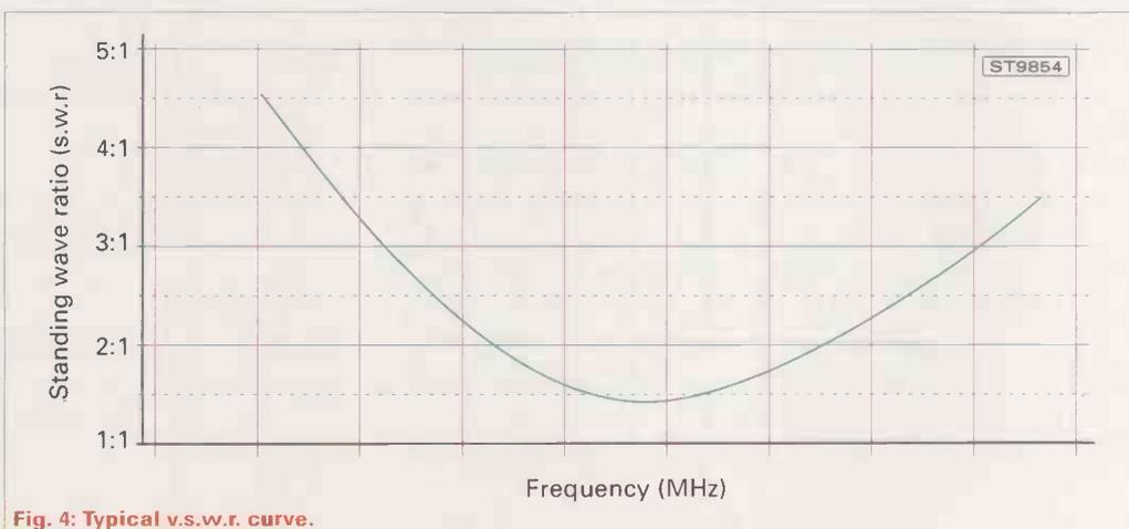
**Fig. 4: Typical v.s.w.r. curve.**
