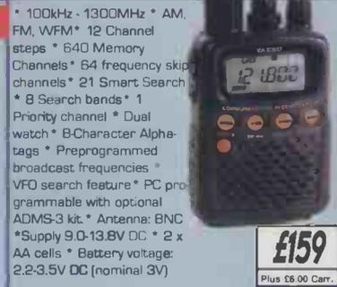
\* 100kHz - 1300MHz \* AM, FM, WFM \* 12 Channel steps \* 640 Memory Channels \* 64 frequency skip channels \* 21 Smart Search \* 8 Search bands \* 1 Priority channel \* Dual watch \* B-Character Alpha-tags \* Preprogrammed broadcast frequencies \* VFO search feature \* PC programmable with optional ADMS-3 kit \* Antenna: BNC \* Supply 9.0-13.8V DC \* 2 x AA cells \* Battery voltage: 2.2-3.5V DC (nominal 3V)
