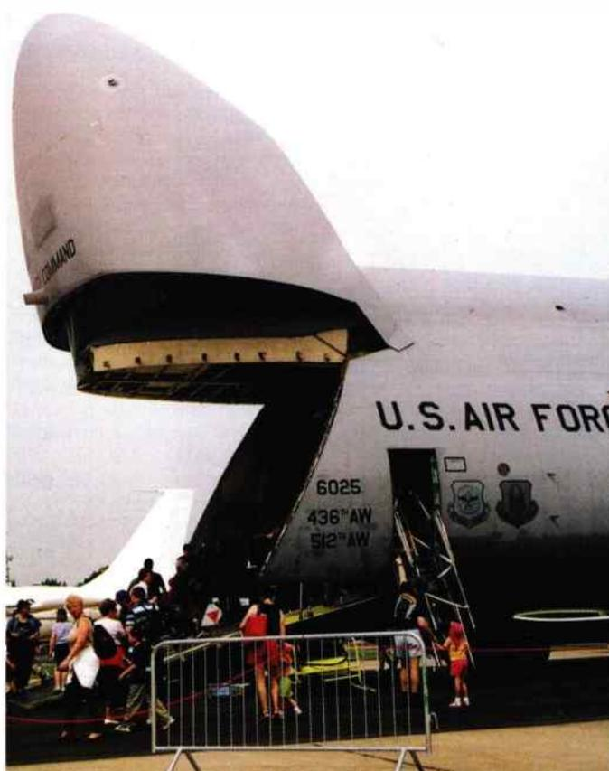
Lockheed C-5B Galaxy at the RAF Mildenhall Air Fete in 2001. The open nose allows out-sized loads to be easily moved in and out. The spectators in the foreground show the massive proportions of the aircraft. (Photo: Graham Tanner).
