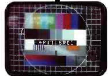
Fig. 3: The FuBK test card radiated in the Seventies by the Swiss +PTT.
