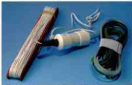
**Graham Tanner's Revco Angler portable short wave antenna. The 45m roll of antenna wire is to the left, and plugs into the balun (top right). From the balun, the signal splits to either the BNC connector (black lead) or crocodile clip (green lead).**
