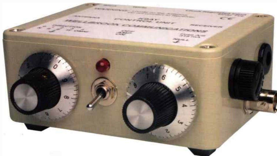
**Null and Direction knobs reside on the front of the K9AY Control Unit. The socket for the p.s.u. end receiver output on the side.**
