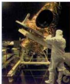
Fig. 1: MSG-1 SEVIRI imager undergoes tests before launch - image courtesy EUMETSAT.
