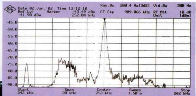
**Fig. 2: The station on 252kHz and its nasty sideband reduced by some 30dB.**
