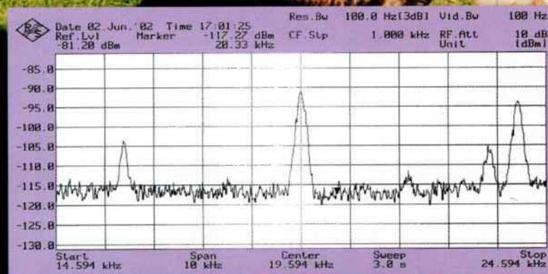
Fig. 6: The signal from Fig. 5 at 20.33kHz significantly nulled.
