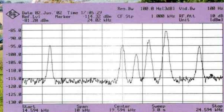
Fig. 5: The spectrum of signals centred on 19.5kHz with the one on 24kHz nulled.
