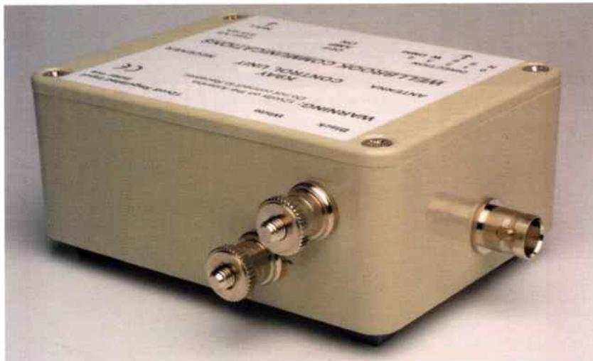
Control wires and antenna feeder connect here.
