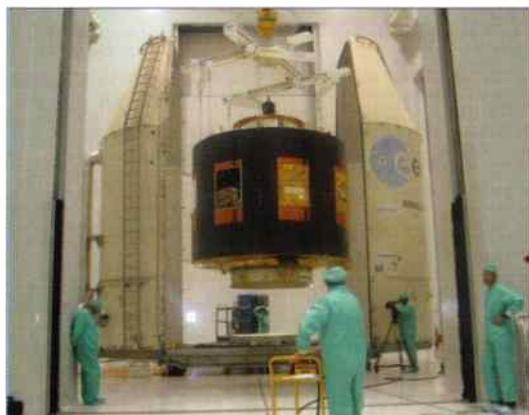
Fig. 2: MSG-1 - courtesy EUMETSAT. On 31 July 2002, the satellite is viewed inside its container in a clean room. After establishing clean conditions in room SSA, the container is opened and the satellite lifted, put out and on the filling stand.
