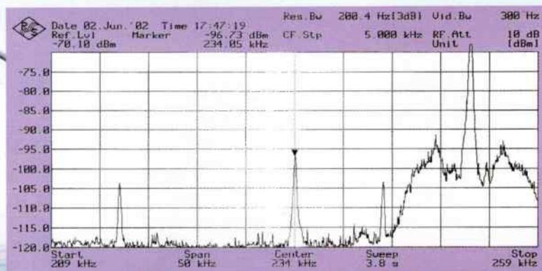
Fig. 4: The 234kHz signal and its sidebands reduced by 26dB whilst hardly affecting the 252kHz station.
