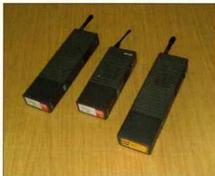
These are the three PFX sets. The middle one is the standard unit. The other two are the sneaky beaky encrypted sets.
