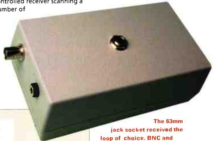
**The 63mm jack socket received the loop of choice. BNC and coaxial power connectors to the rear.**
