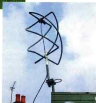
**Fig. 8:** Quadripolar Helix Antenna for a.p.t. reception.
