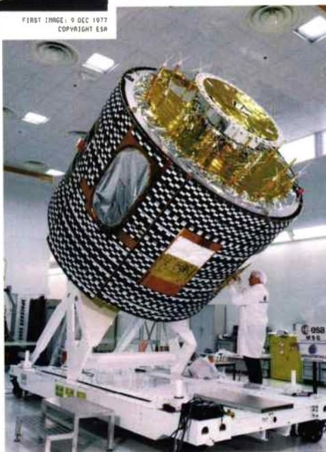
**Fig. 2: The *MSG-1* satellite - Structural and Thermal Model (STM) during the integration and transport to the LSS for thermal vacuum testing at ESA/ESTEC. Image copyright ESA.**
