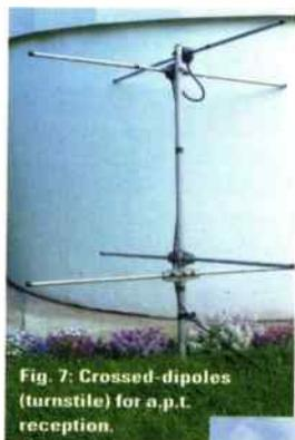
**Fig. 7:** Crossed-dipoles (turnstile) for a.p.t. reception.
