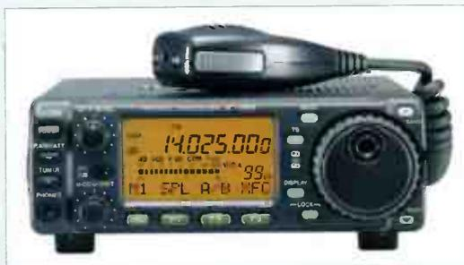
The internal antenna tuner covers from 1.8 to 54MHz. Field and mobile operation are made simple and efficient, especially when using a short antenna covering narrow bandwidth. Latch relays are used for the antenna tuner to greatly reduce the power consumption. The built-in antenna tuner eliminates the need to carry an extra one with you.
