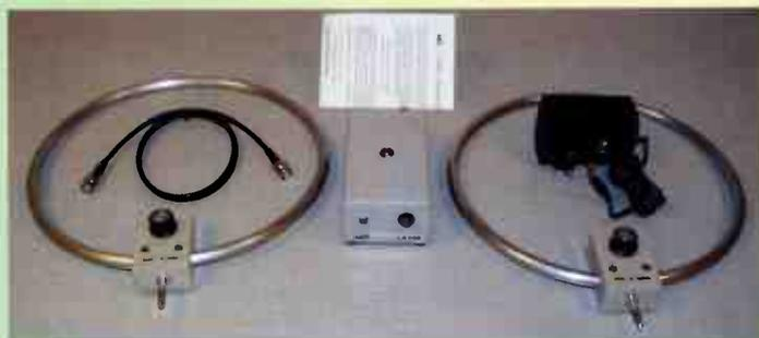
The **WL500** is a compact active loop antenna specifically designed to provide good reception while travelling or operating from a temporary / compromised monitoring location where large external antennas are not practical. The wire loop will fold down and fit into a small bag, operation is even possible using an internal 9V dry battery.
