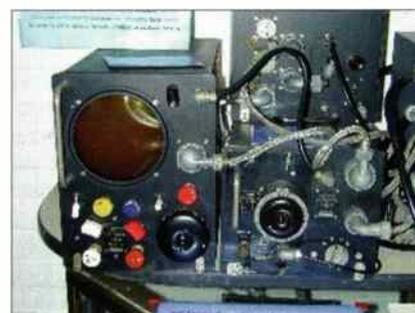
**Fig. 4: The Navy already had access to a system developed by the RAF known as Gee. This was used in the Dieppe raid in 1942 and was later fitted as the standard surface navigation system.**
