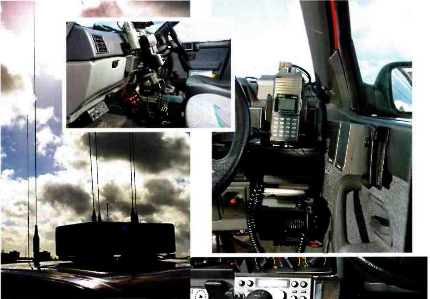
feature, you'll see the various features such as power breakout boxes, which allow rapid temporary installation of ancillary gear. One thing that particularly strikes me is number of external speakers mounted around the car. From my own experiences, I can say that this easily allows the rapid determination of just which radio audio is coming from - though I imagine it takes a while to learn which is which initially.
