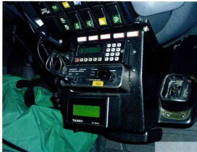
**The rack stack in the ambulance, showing from the top: Yaesu VX-1000 MPT1327 set, then the VXR-2000 repeater set and finally at the base, the display unit.**
