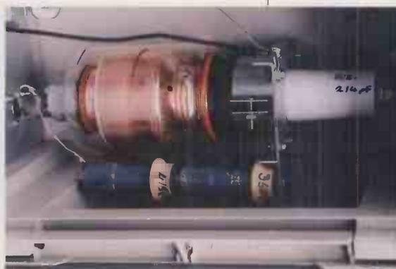
The series capacitance is made up of a fixed value of 200pF and a vacuum variable unit. Perhaps it may seem like overkill for such a modest system, but it does work well.
