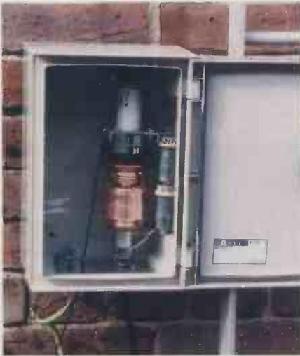
An overall view of the matching unit in the metal security box mounted outside. The coaxial feed and antenna wire pass through base of the box.
