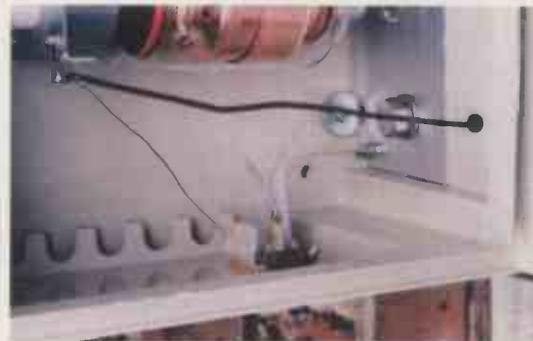
The spark gap fitted to protect against antenna static build-up. The static leak resistance is made up of two 470kΩ (each one of 4W dissipation) resistors.
