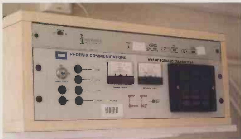
*The Inovonics 222 audio processor, and Phoenix Communications transmitter make a compact pair on the shelf.*
