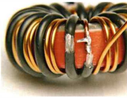
insulation from the wound coaxial cable adjacent to the previously soldered joint to expose the screen.
