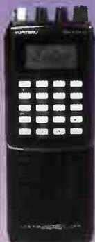
Wideband hand-held scanner covers 500kHz-1650MHz. (All mode). Includes nicad/car charger/charger/antenna. Extremely user-friendly hand-held receiver with outstanding performance unmatched by its rivals.
