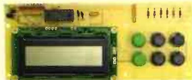
23/24cm version connects to Rx & Tx for easy pushbutton frequency control in 125kHz steps, 3 VFOs, auto-tune Rx to Tx frequency & much more. Enables wideband Rx too!
