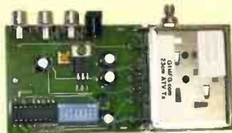
The UK's most popular amateur television transmitter. Transmits high quality pictures and sound anywhere in the 23/24cm band in 500kHz steps, 50mW min. output power (70mW typ).
