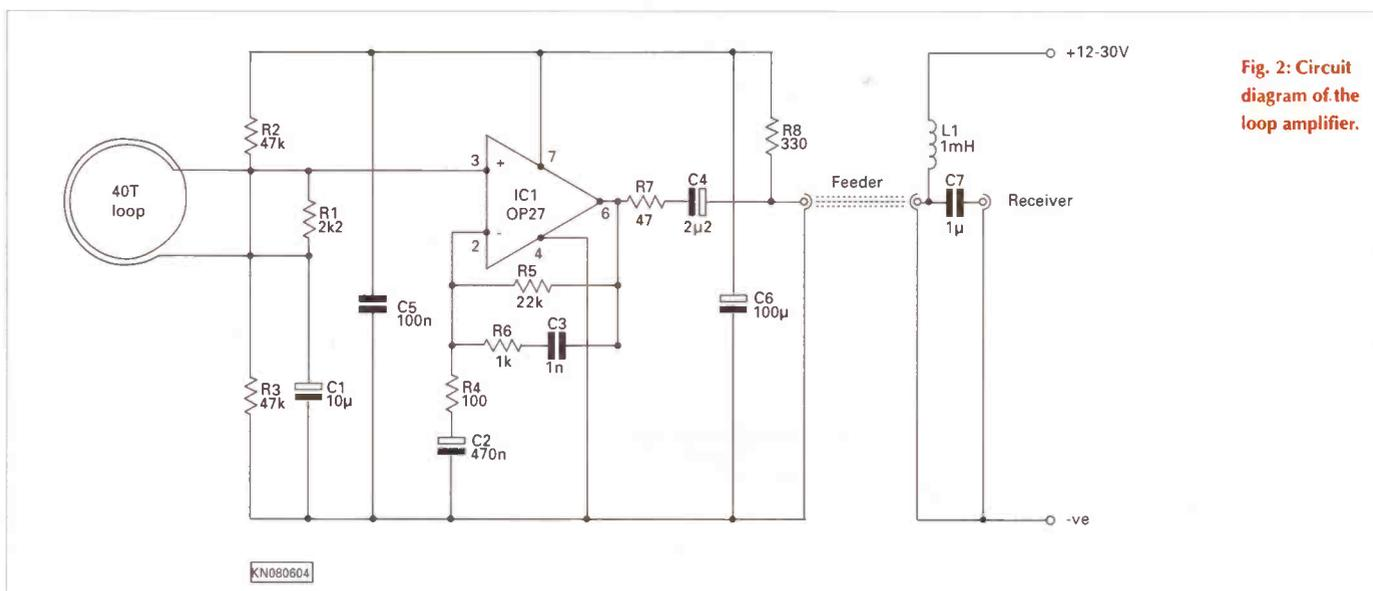
Fig. 2: Circuit diagram of the loop amplifier.
