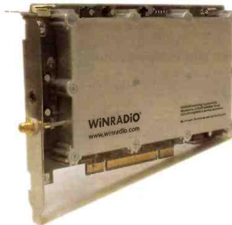
The high sensitivity is also matched by that of the S-meter: The calibrated S-meter shows the received signal levels in dBm,  $\mu\text{V}$  or S-units, down to the receiver noise floor. The IF bandwidth of the receiver is continuously adjustable from 1 Hz to 15 kHz, in 1 Hz steps.
