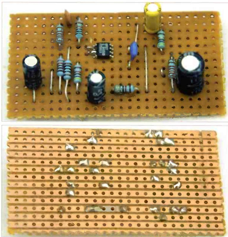
**Fig. 3: The amplifier circuit partially assembled on Veroboard. Note the glued on SO8 version of the OP27.**
