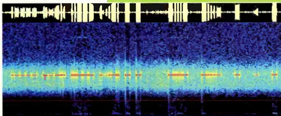
Analysis of M03 transmission - note bandwidth due to filter use.
