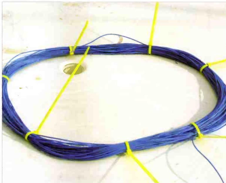
Fig. 1: The loop is wound with 40 turns and has a diameter of 380mm.
