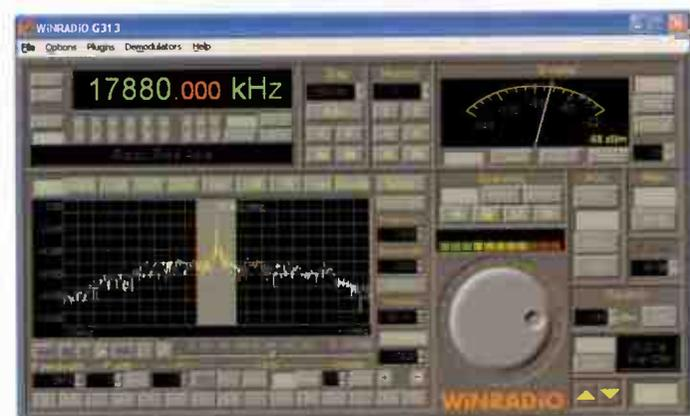
The receiver is extremely sensitive, making it possible to comfortably read CW signals well under -130 dBm input level, yet featuring a respectable 95 dB dynamic range making the receiver resistant to strong signal overload.
