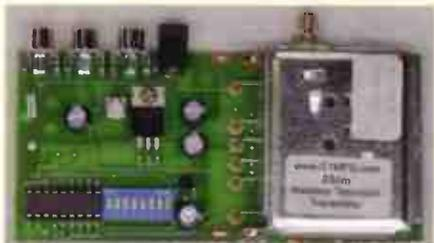
Transmits high-quality pictures and sound (includes 6.0 and 6.5MHz sound subcarriers). DIP switches set the operating frequency.
