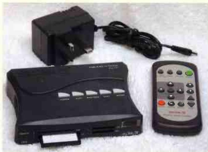
Our new Test Card Generator is supplied with over 20 sample test cards and can hold 100 or more on its Compact Flash memory card – and you can use almost any image editing software to make your own test cards! Very easy to use. Operates from 12V DC. Composite and S-video (Y/C) outputs. Comprehensive set of accessories supplied including mains adapter, remote control, composite & S-video leads. **Amazing value!**
