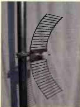
SMA input, with free mast mounting kit. Typically 13dB gain, OK for receive from 2.2-2.7GHz.
