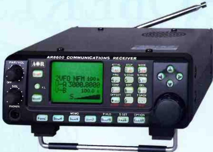
**AR8600MK2** can be used mobile, base or transportable... powered from an external 12V d.c. power supply, 12V vehicle or from an optional internally fitted NiCad battery pack. The upper frequency range is to 3000MHz (3.0GHz), with enhancement to short wave performance. 1000 memory channels, resizable memory banks, alpha text comments for banks and individual channels, frequency pass and lockout, built-in RS232 port, optional slot card available. **£719.00**
