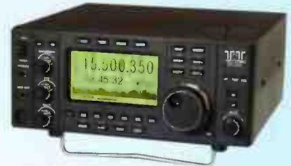
**RX350D** The Ten-Tec **RX-350D** is a full featured, mid-price range HF DSP receiver. Now even more versatile due to the inclusion of the 12kHz I.F. socket on the rear panel for DRM use (demodulation software required). On-screen band activity display adds a new dimension to locating transmissions and tuning the receiver, 34 DSP bandwidths provided, noise reduction etc. **£999.00 inc VAT, UK carriage £10.00**
