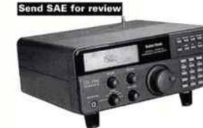
★ Superb performance SW receiver ★ 0.2-30MHz (all mode) ★ Selectable tuning steps (down to 100Hz) ★ 240 or 12V ★ Digital S-meter ★ Attenuator ★ Key pad entry ★ 160 memories ★ Noise blanker.
