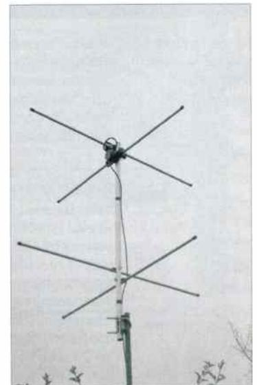
**Fig. 8: 137MHz crossed-dipole antenna (turnstile).**
