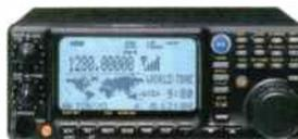
This amazing desktop scanner is the only scanner to offer true dual receive. Coverage is from kilohertz to gigahertz offering all modes and has optional DSP for enhanced shortwave reception.
