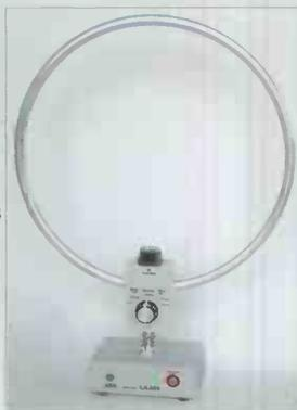
The LA380 is a compact active (30cm diameter) loop aerial specifically designed to provide good reception when away from the main monitoring location or when large external aerials are not practical. Compact, but achieving high performance, featuring an internal high gain amplifier (20dB for 10kHz-250MHz) and excellent overall strong signal handling (high IP3 +10dBm).
