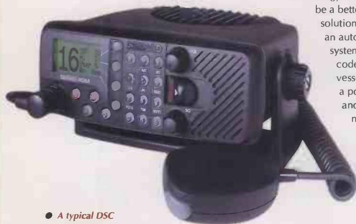
● A typical DSC equipped radio.
