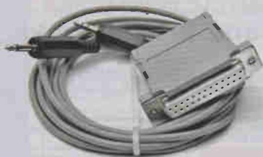
The Pervisell 'SkySpy' interface features a 'pass-through' audio lead that will fit into the Sound Card's input.
