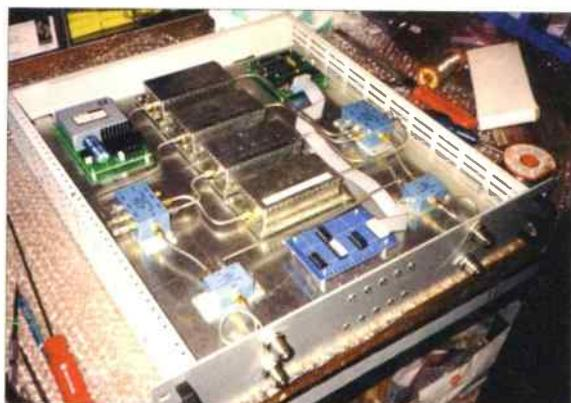
**A signal bandwidth selector unit for the Very Long Baseline Interferometry (VLBI) system at Jodrell Bank.**
