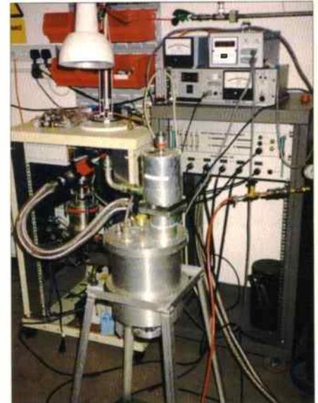
**Testing of a 5GHz receiver used in the MERLIN array of telescopes. The cryostat is cooled with a helium gas refrigeration system to about 15° above absolute zero.**
