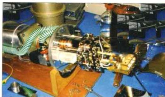
**A receiver cryostat under construction. This is one of fourteen 33GHz receivers which will form part of the Very Small Array (VSA) on Tenerife to study the radiation originating in the Big Bang.**
