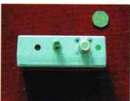
**Fig. 5: Connectors for down-converter.**
