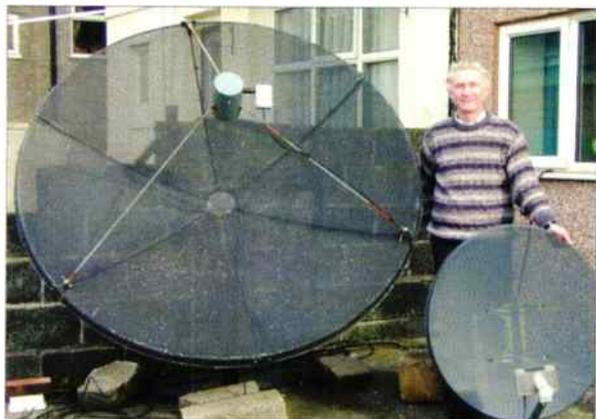
**Fig. 8 (above):** Dishes for METEOSAT PDUS and WEFAX telemetry.
