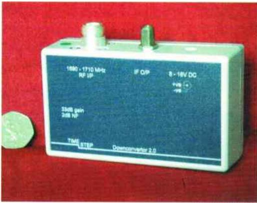
**Fig. 4: Down-converter.**
