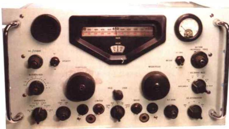
was reckoned to be the best thing around, I was impressed by the design of the RA-17, for here was a receiver with an almost linear frequency readout (which was also accurate), and resettability of a class which I had not seen before (and they told me it was drift cancelling as well!).
