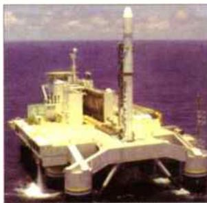
Aerial view of the 'Sea Launch' rocket platform, a modified oil drilling rig. Control operations are from a nearby ship.
