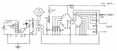
Fig. 1. Circuit of the Combined Instrument. S3 is the change-over switch, selecting either RF or DC measurements. By using an external battery, the resistance range can be multiplied up to ten times.
