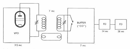
Fig. 2. Block diagram showing tuning sequence with VFO on 3.5 mc. The 7 mc CO becomes a buffer-doubler when, with the crystal removed, it is driven from the VFO. If the original CO was operated on the fundamental of the crystal, the buffer will have to be neutralised unless it is a tetrode or pentode in a stable, well laid out circuit.
