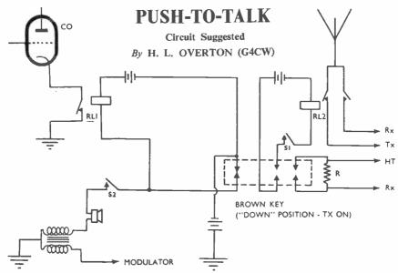
Circuit of G4CW's change-over system. It involves use of a multi-contact key, such as the old Brown, though for telephony working only, a spring switch would give the same result. RL1 is the keying relay, and RL2 the aerial change-over relay; S1 is to save the battery when the station is off the air, and S2 can be the switch in the microphone stand.
