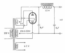
Fig. 3. A well-smoothed separate power supply is an essential for satisfactory operation of the VFO.
