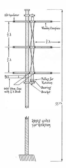
Diagram gives main details of the six-\frac{1}{2}-wave-in-phase vertically stacked 58 mc aerial at G6CW (Notting-ham). All elements are \frac{1}{2}-wave long, with \frac{1}{2}-wave separation, and fed through a 600-ohm line across a \frac{1}{2}-wave matching stub at the base of the array. G6CW credits this aerial with his recent successes on \frac{5}{2}-metres.
