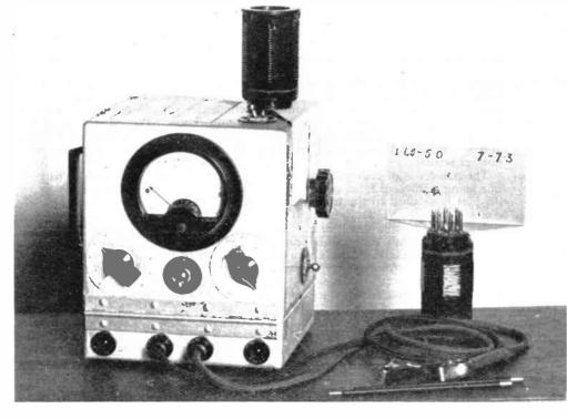
GSBY's V.O.M.-Frequency Meter. General view of an instrument covering 1-35 mc, and giving readings up to 5,000 volts, with current scales to 1,000 mA and resistance readings to 500,000 ohms.
