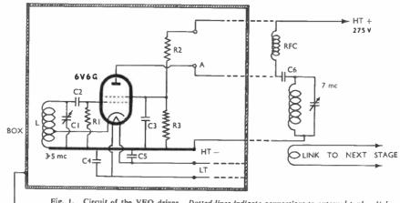
Fig. 1. Circuit of the VFO driver. Dotted lines Indicate connections to external tank. Values are: L, 24 turns 16 SWG enamelled on standard plug-in former, with tap 8 turns from earthy end; C1, 160 \(mu\mu\mathbb{F}\); C2, 200\(\mu\mathbb{F}\); C3, C4, C5, \(01\) \(\mu\mathbb{F}\): C6, \(001\) \(\mu\mathbb{F}\); C8, \(000\) ohms, \(1\) watt; R2, \(50,000\) ohms, \(1\) watt; R3, \(20,000\) ohms, \(1\) watt.
