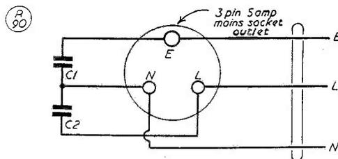
Fig. 7. Additional mains filter to be fitted at plug point. C1, C2 are 2.0  $\mu$ F, not less than 1000v. wkng. The lettering N, E, L, stands for "neutral, earth, live," and should appear on all plugs and sockets in properly-wired installations.
