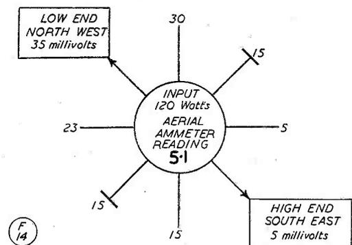
Fig. 2. Some relative field strength readings taken round a 40-metre T2FD operated on 14 mc, at a distance of 500 feet.
