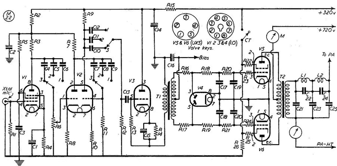
Fig. 1. Circuit of the 807 modulator designed by VK2AWU and discussed in his article. It incorporates speech limiting.
