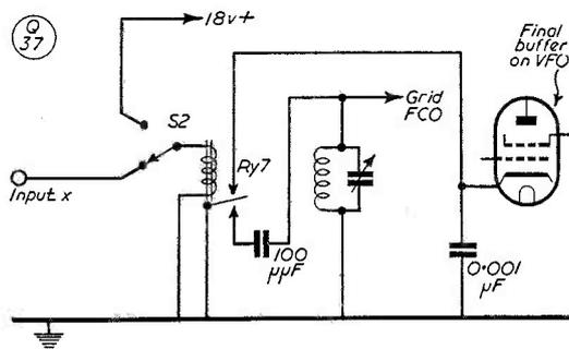
Fig. 2. Control applied to the early stages of a transmitter.
