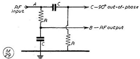
Fig. 1. Basic phasing network, the action of which is discussed in the text.
