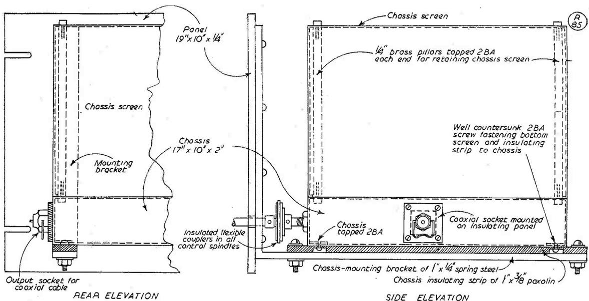
Fig. 2. Sketches showing detail for panel and chassis mountings for the type of receiver discussed in the text.
