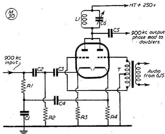
Fig. 2. Practical circuit for phase modulation, with all necessary values in table. The author of the article operates successfully on the 80-metre phone band, using this method of control.
