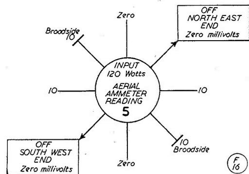
Fig. 4. Field strength readings at 500 feet round a coax-fed horizontally disposed 40-metre cut T2FD operated on 14 mc. This sketch should be compared with Fig. 2, for which the aerial was correctly tilted.
