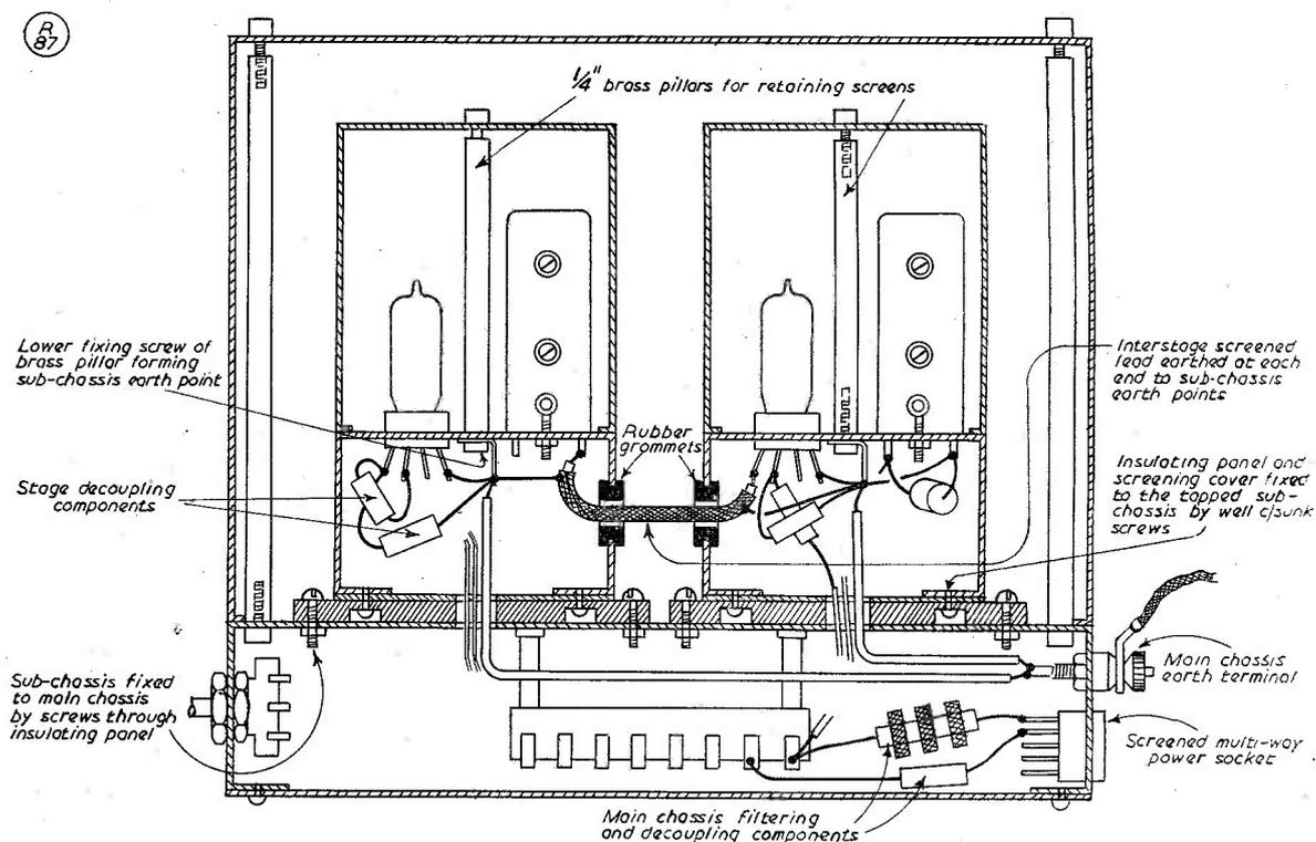
Fig. 4. Cross-sectional view of sub-chassis, showing methods of fixing to main chassis, and general wiring scheme.
