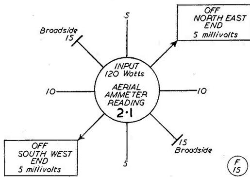
Fig. 3. Relative field strength readings, taken at 500 feet, round a coax-fed 14 mc dipole. Compare with Fig. 2, noting that the transmitter input is the same in both cases.
