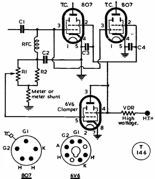
Fig. 2. A PA consisting of a pair of 807's in parallel, a very popular arrangement, in which protection is obtained by the same circuit as Fig. 1. Here again, R1 can be regarded as a variable power control on the screens of the PA. A circuit embodying these principles should be used with all tetrode RF amplifiers.
