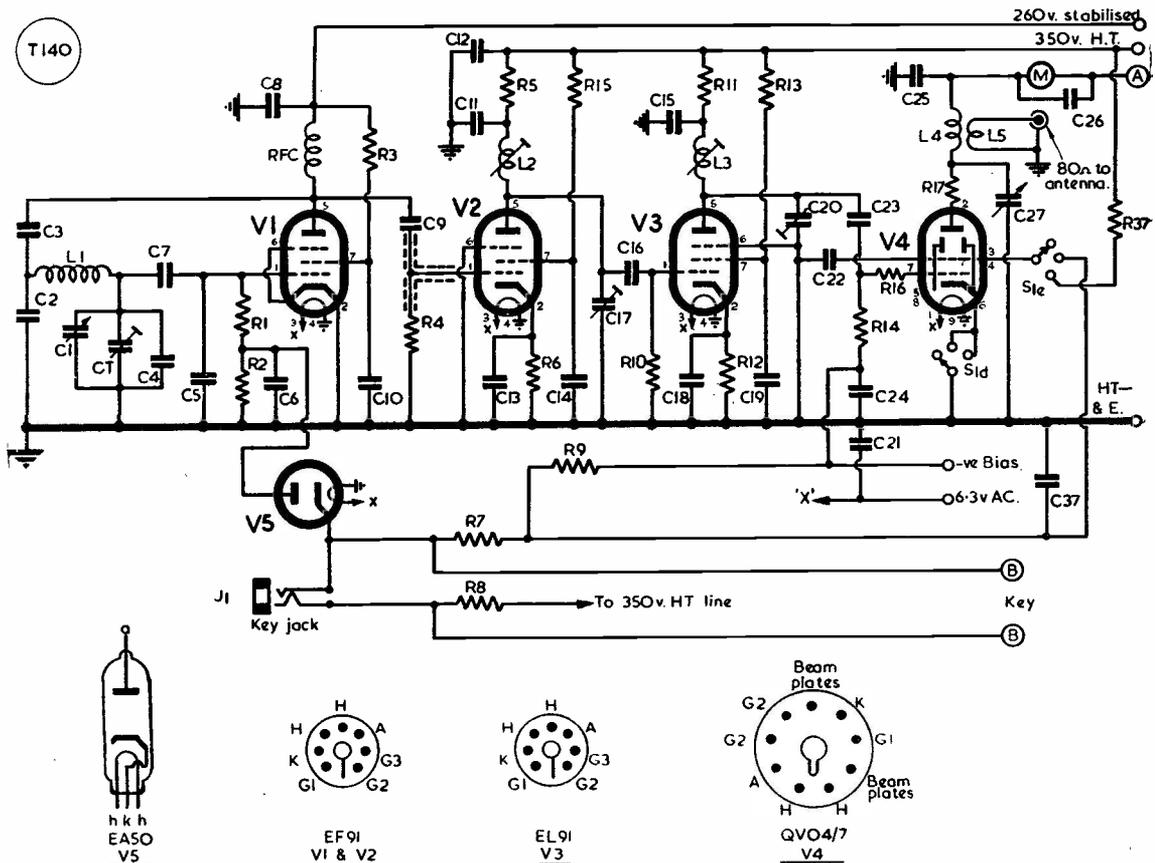
Fig. 1. RF section of the 160-metre transmitter described by G3FRV. It is a straightforward VFO-BA-BA-PA arrangement, designed for full break-in working and relay control on telephony. The VFO features the extremely stable Tesla oscillator circuit, and miniature valves are used throughout this section. The design for the modulator will be given next month.
