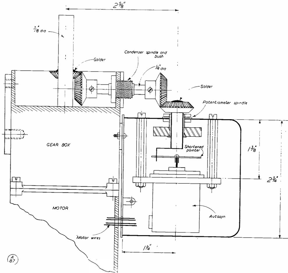
Fig. 2. Showing mechanical arrangement of the Autosyn drive, mounted on the main motor housing at the base of the mast.
