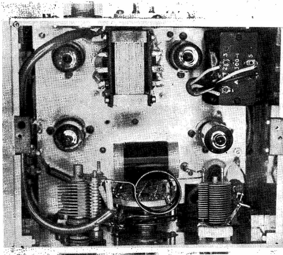
Internal layout of the G2XX all-band transportable transmitter, looking down into the upper section, above chassis. The PA coils are arranged centrally, as near as possible to the band-switch, the PA valve is right front, and the 12AU7-12AT7 modulator section is at the back. All in a 6-inch box, and TVI-proof, too!
