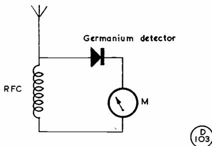
Circuit of the aperiodic radiation meter which, by its very simplicity, can become one of those indispensable items of test gear. The germanium detector and the RF choke are standard items, and can be wired in behind the meter itself (like a shunt).
