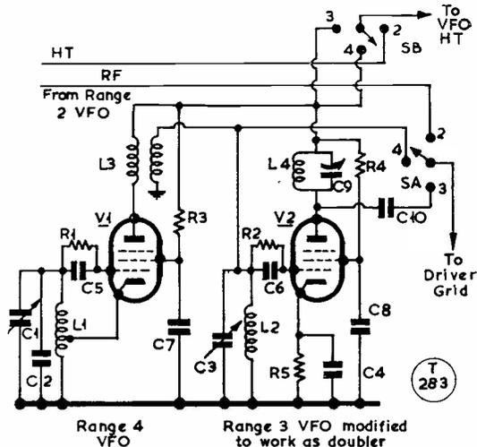
Fig. 1. This diagram shows the circuit of the VFO/doubler combination used on Ranges 3 and 4, in G3BST's TA-12 modification. Considerable simplification is achieved by converting the Range 3 VFO to work as a doubler, as explained in the text.
