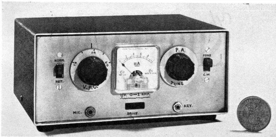
How the miniature mobile Tx, as designed and constructed by G3SRY, looks when completed — note the half-crown for size comparison. The PA consists of a pair of Mullard AUY10's, running the full 10 watts input on 160m. from a 24-volt supply line, loading to just over 400 mA. The design incorporates VFO control, and high-level modulation is by another pair of AUY10's — see circuitry.
