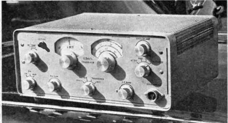
Shown at the Barford Rally — the very fine 20-80-160m. Sideband transceiver built by G3HVX (Hereford). Beautifully constructed, it has a separate dial (left) for the IF incremental tuning control on the Rx side; this enables the receiver to listen off the Tx frequency. *A G3GMN print.*
