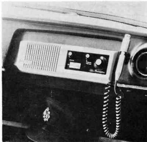
A commercial mobile installation as supplied by Rediffon Telecommunications to the Nigerian Police Force. A 100-watt SSB set for HF working, it has been tested under location conditions to give ranges up to 900 miles or so.
