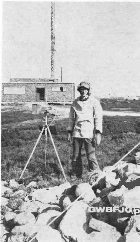
The three-centimetre rig operated by GW8FGP/P, running 10 mW with a Gunn oscillator and using a horn antenna giving about 22 dB of gain. See notes on p.397, September issue, and the narrative.
