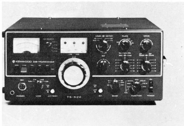
The TS520—latest in the new TRIO line of superior amateur radio equipment. Its styling and finish put all other rigs in the shade; and it is not just pretty—the front panel is a die casting giving unheard of strength and stability.
