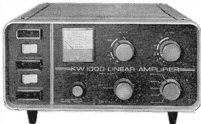
Decca KW 1000 Linear Amplifier for SSB and CW 10-80 metres, 1200 watts p.e.p. input SSB, can be "driven" by most 100 watt Transceivers and Transmitters. Employs a pair of T160L Tubes in grounded grid. Pi-section input and output circuits. Built-in 2-4K P.S.U.
