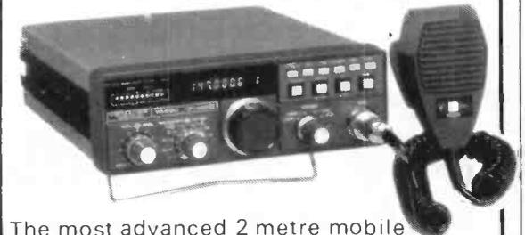
The most advanced 2 metre mobile available today - USB, LSB, FM, CW full scanning with priority channel, 4 memory channel, dual synthesized VFO system.
