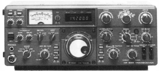
A recent addition to the Trio HF range, and proving amazingly popular is the new TS530S. Designed as a "little brother" to the TS830S, the TS530S uses the same PLL system, same RF boards, same readout system and many other features of the 830 but without the variable bandwidth facility. You do, of course, have the famous Trio I.F. shift system for dodging the QRM.
