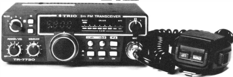
The TR-7730 is an incredibly compact, reasonably priced, 25-watt, 2-meter FM mobile transceiver with five memories, memory scan, automatic band scan, and other convenient operating features.
