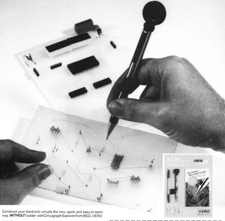
With Easiwire all you do is wind the circuit wire tightly around the component pins. No soldering, no chemicals, no extras, simplicity itself. Circuits can be changed easily, and components re-used.
