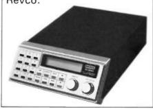
onto each channel which is a bonus because some costlier scanners only allow delay to apply to all channels or none, not individual ones.
