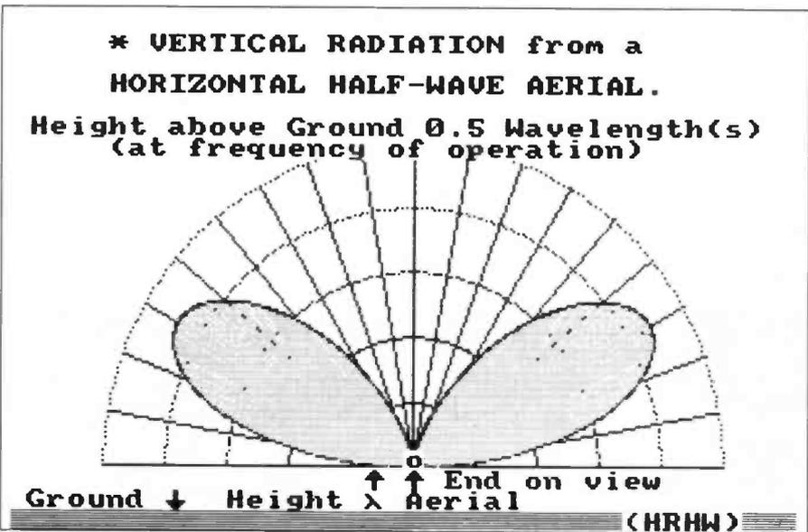
Fig. 2.7: As Fig. 2.5, but for an electrical height above ground of  $\lambda/2$ . See text for details.
