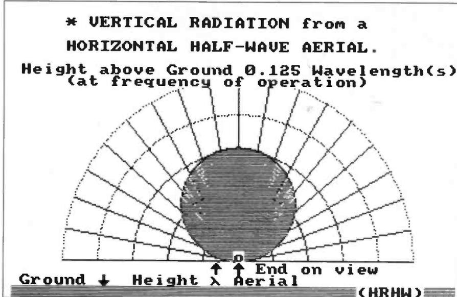
Fig. 2.5: Vertical radiation pattern for a  $\lambda/2$  antenna at an electrical height above ground of  $\lambda/8$  at operational frequency.
