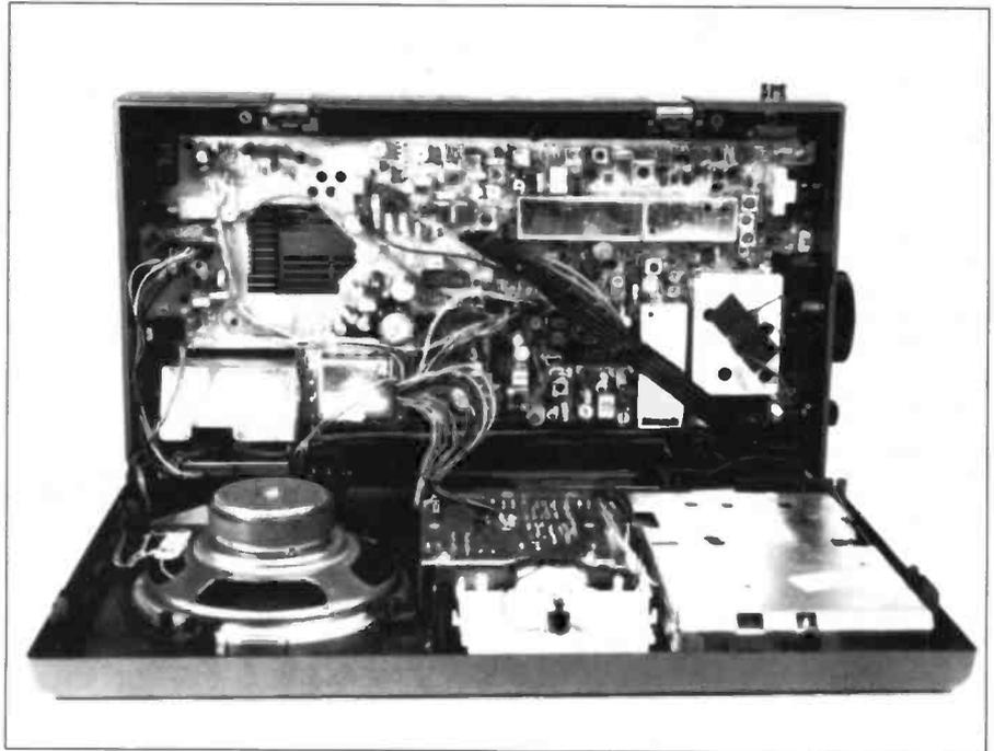
For the utility station enthusiast the International 400 is fitted with a variable beat frequency oscillator (b.f.o.). This is essential for resolving c.w. and RTTY, etc. The b.f.o. is only available on short wave and is operated by pressing a small button on the right hand edge of the radio. The tuning for the b.f.o. comprises a 12mm diameter knob also on the side panel, which turned out to be quite easy to use.
