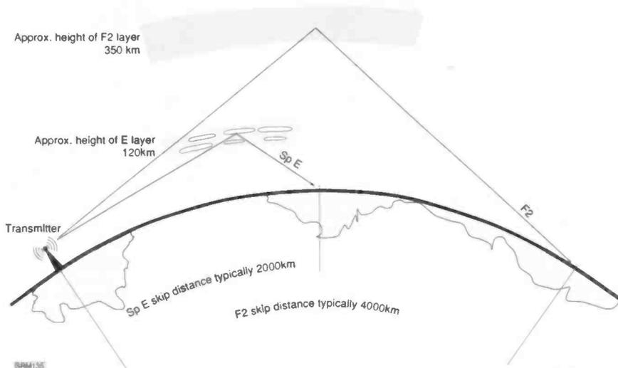
Fig. 1: Comparison of skip distance between sporadic-E and F2 layer propagation.
