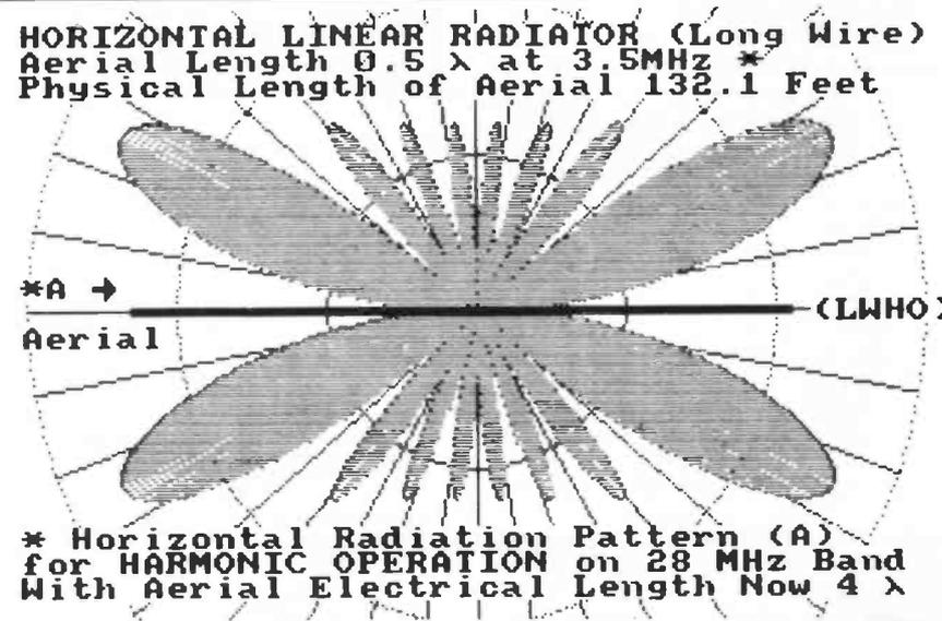
Fig. 2.4: As Fig. 2.2, but for harmonic operation at 28MHz (8 times the fundamental).
