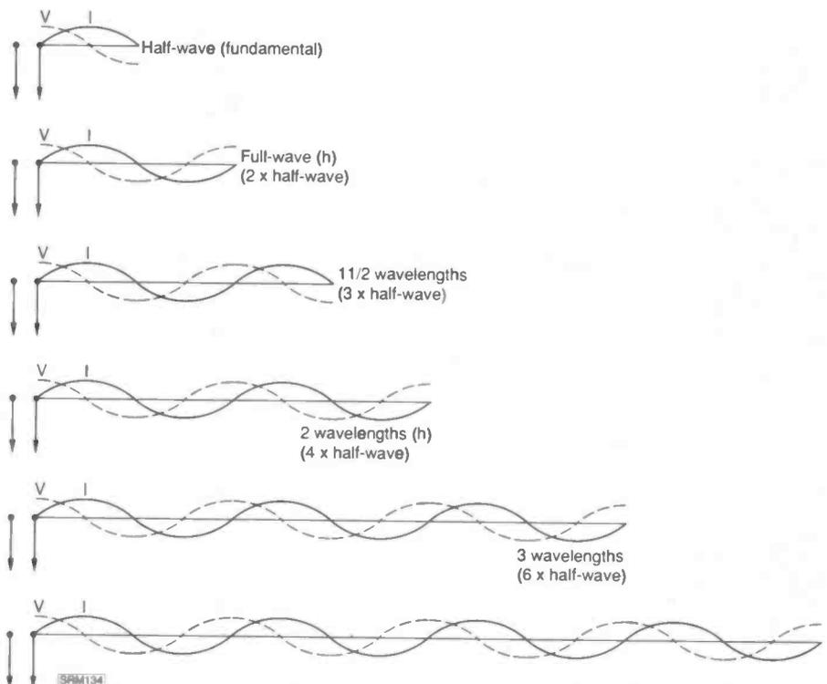
Fig. 2.1: Current and voltage distribution for a linear antenna operated at a fundamental frequency, or at frequencies harmonically related to a fairly low fundamental frequency, e.g. 3.5MHz.
