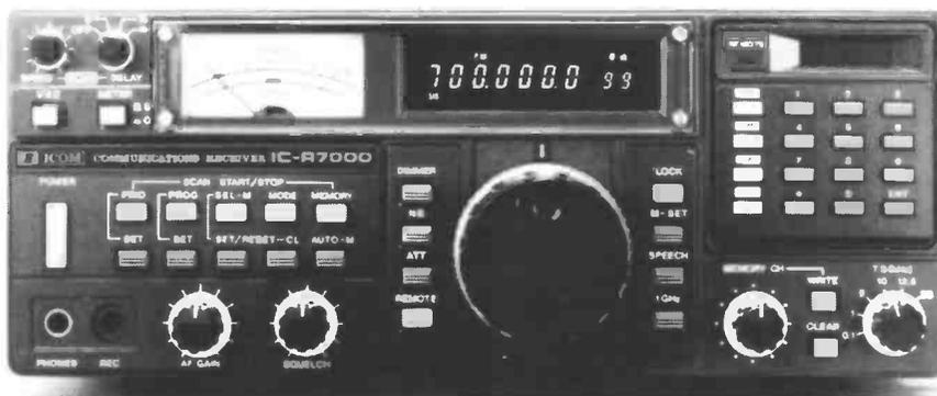
ICOM introduces the IC-R7000, advanced technology, continuous coverage communications receiver. With 99 programmable memories the IC-R7000 covers aircraft, Marine, FM Broadcast, Amateur Radio, television and weather satellite bands. For simplified operation and quick tuning the IC-R7000 features direct keyboard entry. Precise frequencies can be selected by pushing the digit keys in sequence of the frequency or by turning the
