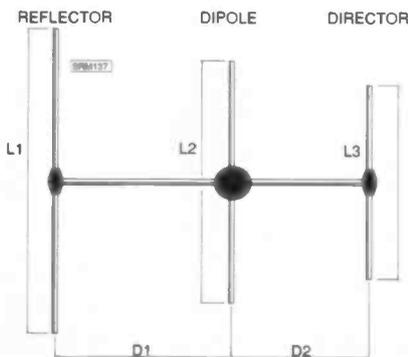
Fig. 3: 3-element array for 45-46MHz vision reception.
