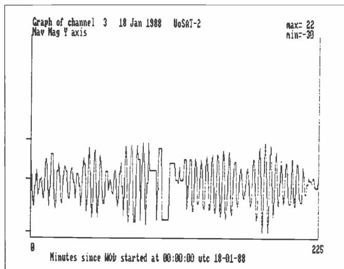
Fig. 2: Graphical plot of the navigation magnetorque Y-axis during part of an orbit in January 1988.
