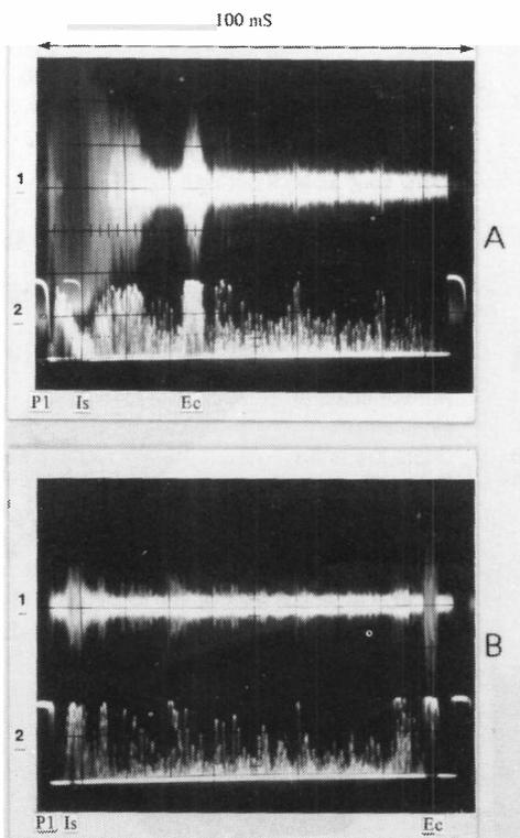
Fig. 3: (A) Upper trace 1. P1 - transmitted pulse. Is - Ionospheric scatter. Ec - echo. Lower trace 2. Rectified versions of the signals (and noise) (B) Upper trace 1. P1 - transmitted pulse. Is - ionospheric scatter. Ec - echo at 90ms (see text).
