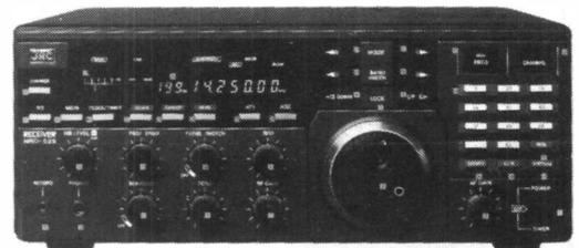
The **NRD525** is a high-class, general coverage receiver with expandability looking to the future. Combining traditional technology unique to JRC with the most advanced digital technology gives superb performance whilst remaining extremely easy to use. The NRD525 covers 90kHz-34MHz and with an optional VHF/UHF converter also covers 34-60, 114-174 and 423-456MHz. Modes of operation CW, SSB (USB/LSB), AM, FM and RTTY with
