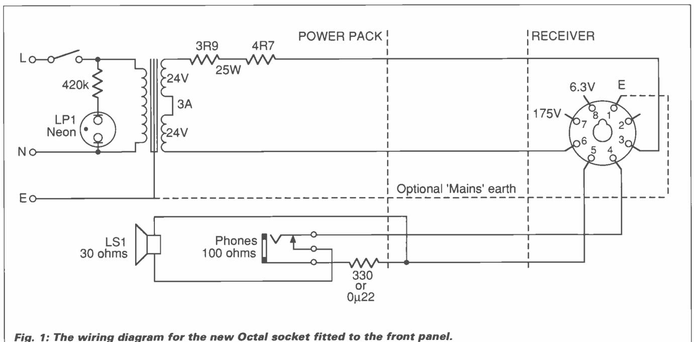
Fig. 1: The wiring diagram for the new Octal socket fitted to the front panel.
