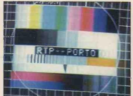
Fig. 2: Portuguese FuBK test card which occasionally displays the identification 'RTP-LISB 1'.
