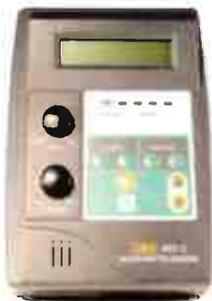
ARD2 portable ACARS & NAVTEX decoder & display unit, can be operated from internal batteries or external d.c. supply. An RS232 port expands capabilities, **free supporting software** from the AOR internet web site.
