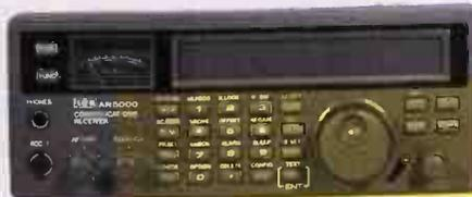
Covering an extremely wide frequency range and offering USB, LSB, CW, AM, FM. It features 1,000 Alphanumeric Memories \* 45 Channels per sec Scan Speed \* 2,100 programmable Pass Frequencies \* DTMF Decoder \* RS-232 Port \* 1Hz tuning steps \* 6 switchable bandwidths \* Preamplifier \* Duplex monitoring \*
