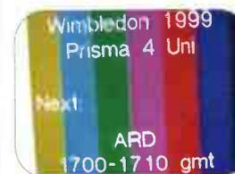
**Intelsat 27.5°W and the BT Wimbledon digital feeder into Europe. Note the unusual colour bars with the white bar right hand side, this is to assist line blanking measurement.**
