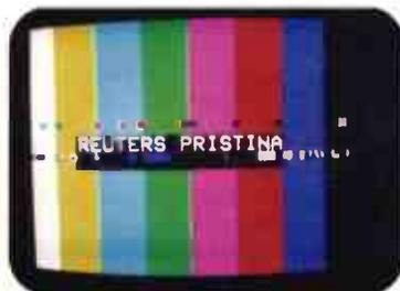
A marginal signal level showing digital threshold breakup (pixellation) on a Balkans feed.
