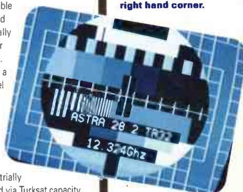
**Astra is all digital at 28.2°E, that is except the analogue test card as a rapid dish orientation aid!**
