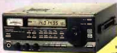
The FRG-100 has stood the test of time. It offers full coverage of the short wave bands plus long wave and medium wave. It features, \* USB, LSB, AM, CW,
