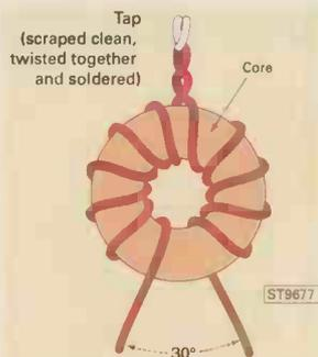
Fig. 1.3: Toroid winding.
