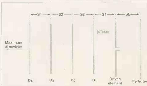
**Fig. 1.4: Six-element beam.**
