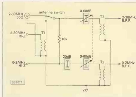
**Fig. 1: R-1000 input circuit.**
