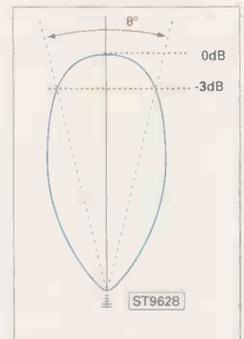
**Fig. 1.2: Antenna pattern beam width is measured as the arc**
