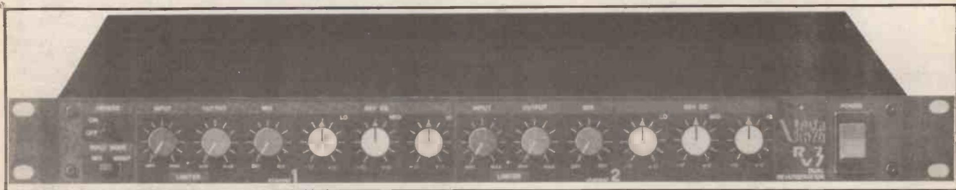
VESTA-FIRE RV-3: a genuine two-channel spring reverb unit which could be a real asset in home recording if used with care
