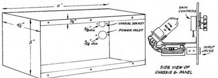
Fig. 1.-Left: The mixer case. Right: Side view of chassis and panel
