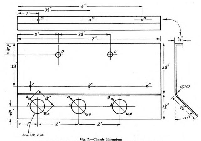
A=holes  $\frac{1}{4}$  in. diam.; B=holes 6 BA clear; C=holes for fixing tag boards (see text); D=holes  $\frac{1}{4}$  in. diam.
