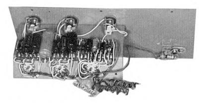
Rear views of the mixer chassis. Top: positions of valves and potentiometers. Bottom: underside, showing component layout
