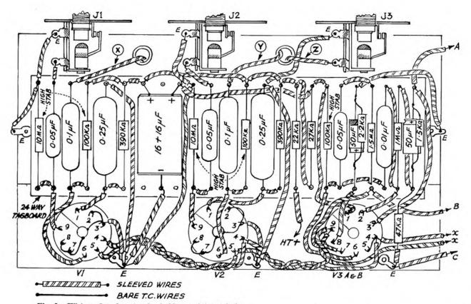
Fig. 3.—Wiring of tagboard valve-holders and input jacks E = solder tags and points earthed to chassis. For all other symbols, see text
