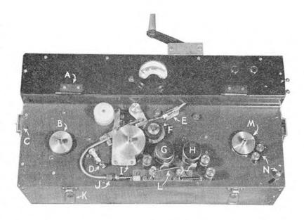
Fig. 1.—The tape deck
