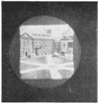
Untouched photograph showing the results obtained using the AM system. Slight distortion of the vertical lines is caused by wow in the tape recorder
