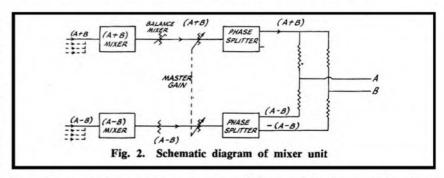
used for each side, and the second half of each valve is used as a phase splitter. This is the familiar split load phase splitter, with equal anode and cathode load resistors. In block form the circuit is as Fig. 1.
