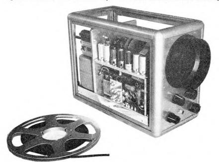
The author's tape "reader" unit, which is capable of accepting either AM or FM signals and provides a long persistence display on a cathode ray tube screen
