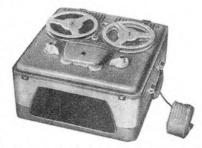
The quoted frequency response was 50-12,000 cps at the top speed of  $7\frac{1}{2}$  ips. Its second speed, 3<sup>1</sup>/<sub>4</sub> ips, had a response of 60-8,000 cps.
