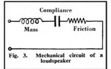
Consider now an alternating force of constant magnitude applied to the weight. At very low frequencies, the velocity of the weight will be limited by the stiffness of the spring and the increase in velocity will tend to be proportional to the increase in frequency.
