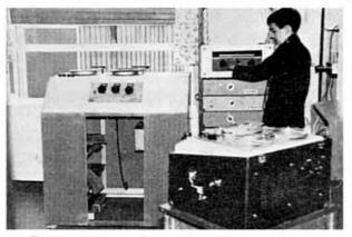
Geoffrey Rivers at the amplifier rack. In the foreground is the E.M.I. TR51 D, and left, the schoolbuilt console housing a mixer and two grams
