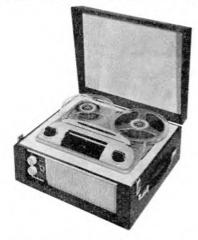
volume control is at the best setting, you pull down a tag marked "R" on the start key, and you are recording.
