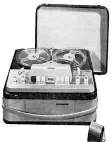
sary socket connections. The playback output from this socket is at a fixed level, and must be controlled on the external equipment. The record input is controlled by the radio/gram level control. The input impedances are: "diode" 0.02 megohm, at a level of 3 mV; record player 0.5 megohm, at a level of 150 mV; and microphone 1,000 ohms, at a level of 1 mV. In addition to the diode output, three other output sockets are provided.
