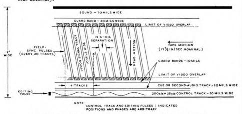
Arrangement of tracks for video tape-recording (405 line standards)
