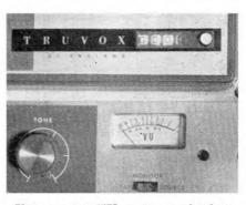
Very accurate VU meters are fitted to the entire Truvox range. The monitor switch (bottom) provides instant flat response comparison between source and tape signal
