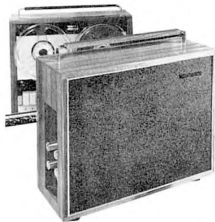
Designed for vertical operation, the VR4 features an eight-inch round loudspeaker with a one-inch coil, which faces to the rear of the machine. Other features include facilities for mixing, meter recording level indicator, parallel track playback, monitoring on track one whilst recording on track three, superimposition, and straight-through amplification, three-digit rev. counter, and separate bass and treble tone controls.
