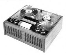
Each machine has two acoustically matched loudspeakers size 7 x 4 inches built-in, and the claimed frequency response is from 30 to 17,000 Hertz plus or minus 3 dB at 7½ ips. Signal-to-noise ratio is claimed as better than 48 dB on the R 52, 46 dB on the R 54. Equalisation is to the new CCIR standard and outputs are provided at external speaker sockets to give 6 watts into 8 ohms.
