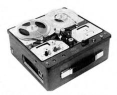
Tape speed is  $7\frac{1}{2}$  ips and flutter is claimed to be 0.1 per cent RMS. Maximum spool size is 7 inches and frequency response is claimed to conform to BS 1568:1960.
