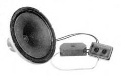
Impedance is now 8 ohms, making the unit particularly suitable for all types of transistorised amplifiers. The mass of the LF diaphragm assembly has been increased to improve bass response in small enclosures. The improvement at the lower end is said to be approximately half an octave down for a given size enclosure relative to the older units.
