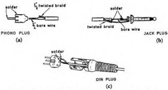
Fig. 2. How to solder screened cable to, (a) phono plug, (b) jack plug, (c) DIN plug
