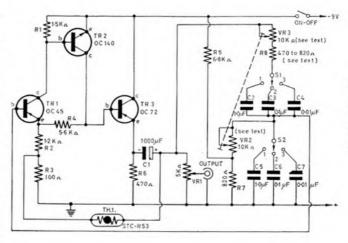
Fig. 1. Circuit for a transistorised audio range sine-wave generator (reproduced from "Circuits for Audio and Tape Recording" by F. C. Judd)
