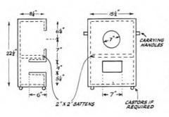
Fig. 4. A design for a transportable monitoring loudspeaker based on the Goodmans Axiette 8 drive unit. Note the strengthening battens; use paint or Formica finish to give the hard wear needed for working in the field. Total building cost around £3 plus the drive unit. (Axiette 8 price price £6 19s. 7d.)
