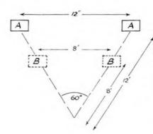
Fig. 2. Stereo loudspeaker pairs AA and BB subtend the same 60° angle and so will produce the same stereo spread at the distances shown. The further away the listener sits the greater must be the speaker separation.
