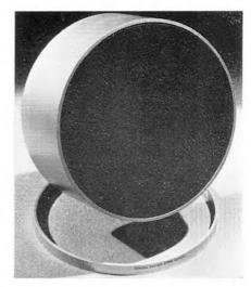
The specification quotes a frequency response of from 50 to 15,000 Hertz plus or minus 2 dB and 50 to 18,000 Hertz plus or minus 5 dB. Power handling capacity is said to be 10 watts continuous—20 watts music power. Impedance is 8 ohms at 1 kHz and construction is of solid aluminium.
