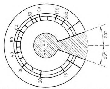
Fig. 2. Calibration of the audio generator. This dial is reproduced here full size and could be cut out and used with reasonable accuracy (from "Circuits for Audio and Tape Recording" by F. C. Judd)
