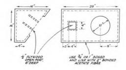
Fig. 3. This design for a wall-mounted monitoring loudspeaker is based on Celestion 12inch drive units. Total building cost of the cabinet work should be about £5 plus the cost of the transducer. (Celestion 2012 price
