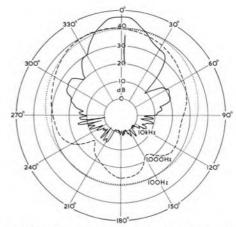
Fig. 1. This diagram shows the polar response of a typical loudspeaker. It will be noted that the high frequencies tend to be concentrated along the axis. Since it is the higher frequency range that conveys a sense of direction to the listener—particularly important in stereo—it follows that both direction and quality will be impaired if the listener is too far off axis
