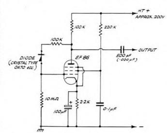
Fig. 3. A simple circuit for a white noise generator for home construction. White noise is an important component in "manufactured" music and sound effects
