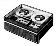
Model M 201 de luxe, an updated version of the M201 series, is a four track single speed (3¾ ips) mono machine. Taking spools up to a maximum of 7 inches in diameter the wooden cabinet is fitted with a strong Plexiglass cover. Frequency response is claimed as 60-13,000 Hertz and wow and flutter better than 0.20%. Signal-to-noise is quoted at 46 dB and the output power is said to be 2.5 watts. Recommended retail price of the M 201 de luxe is 49 guineas.
