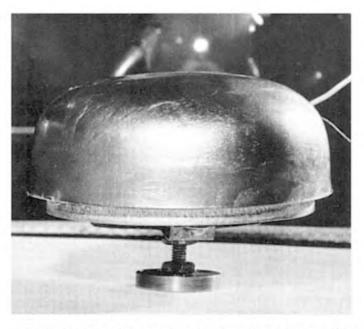
A close-up of the Capsule with a telephone in the background to indicate scale. It can be fixed to any surface, other than marble or solid concrete, and is then claimed to "make music" over the entire area.
