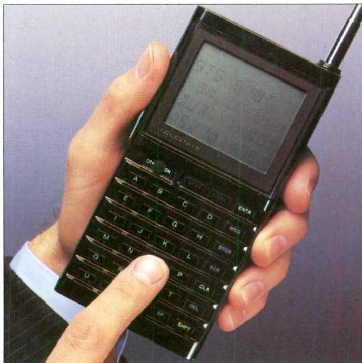
**Left:** Using spare capacity on the VHF/FM frequencies allocated to ILR in London, Radio teletext services can provide the latest financial information from the City, via a hand-held receiver.
