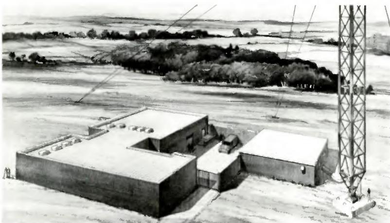
An artist's impression of a building design for a high-power television transmitting station. Once the equipment has been installed such a station will operate automatically under the supervision of a control room many miles away.
