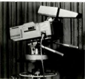
Pedestal-mounted colour cameras used in the studios and for normal outside-broadcast operations.
