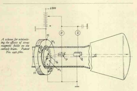
through which the beam passes after leaving the filament. The apparent size of the wire (i.e., the electric field surrounding it) alters with the applied signal voltage. This in turn cuts out a larger or smaller slice S from the centre of the beam B, and so varies the intensity of the light produced by it on the screen.-(Marconi's Wireless Telegraph Co., Ltd.)
