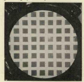
Undistorted image from corrected image tube showing the effect of electrostatic focusing.
