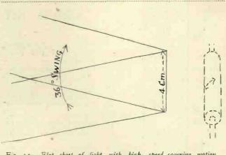
Fig. 12.—Flat sheet of light with high speed scanning motion translated into its own plane.
