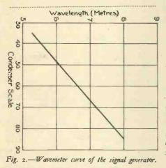
current. The actual point of resonance of the oscillator with the wavemeter is when the anode current is at its lowest. Having obtained the reface, and was built for use as a wavemeter, though provision was made (by including a jack, as shown in Fig. 3a), so that a pair of 'phones could be plugged in if desired.
