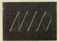
Fig. 3.—Increasing the length of the line by increasing the bias applied to the relay.
