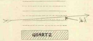
Fig. 3.—Oblique passage of light ray between supersonic wave crests.
