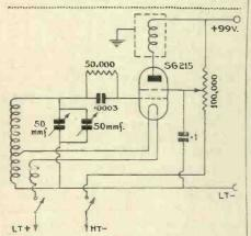
The choke in the positive lead is of a special type obtainable from Eddystone.
