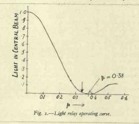
is inversely proportional to this wavelength, being given, in radians, by the ratio of the effective wavelength of light to that of the supersonic waves. (For the first order spectra.) Unfortunately a limit is set by the fact that high-frequency waves in liquids travel
