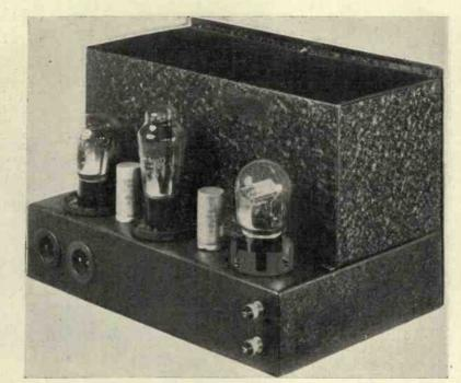
Fig. 7.—On the right is the triode amplifier followed by pentode modulator and balf-wave rectifier. The first two terminals are for the microphone or pick-up input, the first set of sockets for mains input, and the second set for a monitor speaker.
