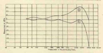
Fig. 36.—Frequency characteristics of the amplifier shown by Fig. 35.
