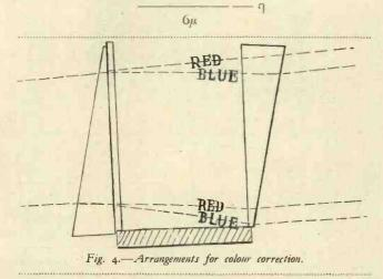
Now the retardation of an optical wavefront produced by a body of thickness T is  $(\mu - I)$  T
