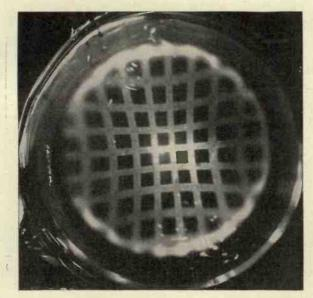
Showing image distortion in uncorrected tube. Comparison with picture showing corrected image tube indicates how focusing is accomplished.
