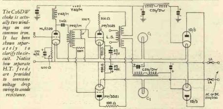
at 50 cycles and .5dB down at 15,000 cycles. This is, of course, *including* the output transformer. If the Baker loud-speaker is not used the bass response can be levelled up as previously suggested by the use of a 200-mfd. condenser across the cathode bias resistance.
