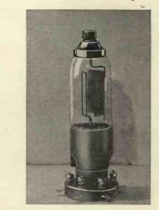
A small type of caesium photo-electric cell. This has a plate cathode and is suitable for televising films.
