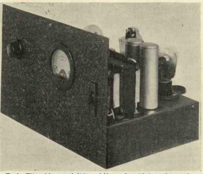
Fig. 6.—This modulator uses the high potential heater values, while the actual output value is a pentode giving between 3 and 4 watts on either A.C. or D.C.
