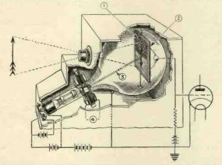
Sketch showing the general construction of the Iconoscope and its method of operation. The reference letters are: 1, Mosaic; 2, Signal plate; 3, Electron Leam; 4, Deflecting coils.
