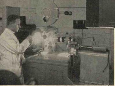
vacuum, photo-electric cell and A & B amplifiers in the large consoles. Below the projector box contains automatically controlled vacuum and water cooler pumps. Below the amplifier is the all-mains supply unit and behind the switchboard are the controls and sound panel. The photograph below shows the transmitter in greater detail.
