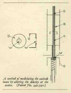
ode-ray receiver-and so producing " streakiness "-the intensity of the beam is varied by altering the density of its centre, whilst leaving the outer diameter constant.
