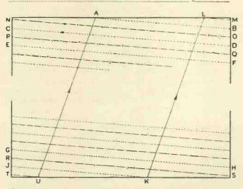
Diagram explaining the method of interlaced scanning employed by the E.M.I. system at the Alexandra Palace.
