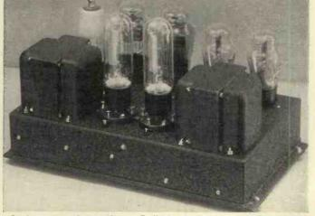
In the centre can be seen the two C1 Philips barretters. Resistances which plug in to valve holders can be used in place of the barretters which require the normal valve holder fittings.
