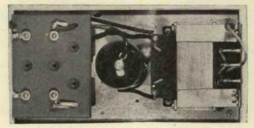
A plan view showing the tappings on the insulated block.
