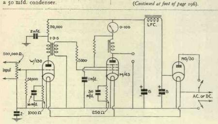
Fig. 8.—This circuit is quite conventional, but has proved very satisfactory with the high voltage values. Notice how the heaters are wired in parallel.
