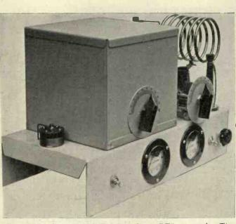
Fig 1. The oscillator provides ample drive for the RFP-15 pentode. The resistance across the modulator input has a value of 1,000 ohms. Although satisfactory results can be obtained with only 250 volts, 500 volts must be applied to obtain 15 watts input.
