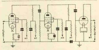
Fig. 35 .- A circuit of pentodes in cascade followed by an output valve.
