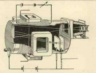
Cut-away sketch showing the internal arrangement of the electron-image camera and its method of operation.
