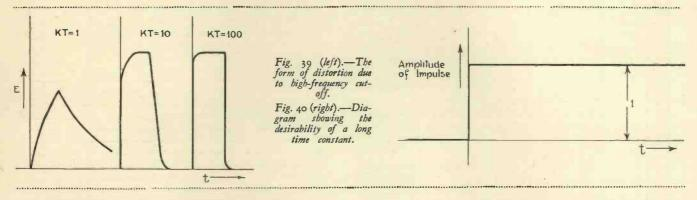
A Rule is given in an article by G. D. Robinson\* that the variation of the amplitude of the flat-topped alternating current component of the picture signal will not
