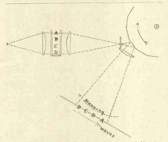
Fig. 1.—Diagram explaining simultaneous production of fif.y picture details on the receiver screen.
