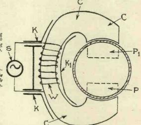
quite satisfactory for the framing frequencies, which are relatively slow; but in the case of the more rapid linescanning frequencies difficulties arise on account of eddy current losses in the magnetic system.
