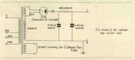
difference that in this case the H.T. voltage is much higher and approximates 3,500. A warning is therefore necessary that the greatest care the leads are adequately insulated, is essential in wiring and insulation there will be no risk in its use.
