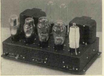
Valves are from left to right two ID5 half-wave rectifiers, two PP3521 triodes, and an HL1320 medium impedance triode.
