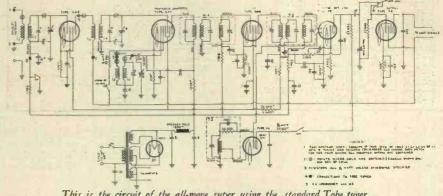
This is the circuit of the all-wave super using the standard Tobe tuner.
