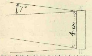
Fig. 10.—Explanatory diagram in plane perpen dicular to high speed scanning motion.
