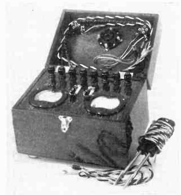
*The complete "Teletester" in its compact box with the accessories mounted in the lid. The testing handles are shown at the side.*
