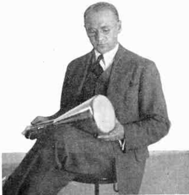
Some time ago our columns gave details of a cathode-ray television receiver, to which reference is made by our correspondent, Mr. Royds. Here we see Dr. Zworykin and his new cathode-ray tube, which he calls a "kinescope." The television images appear on the round flat end at right.
