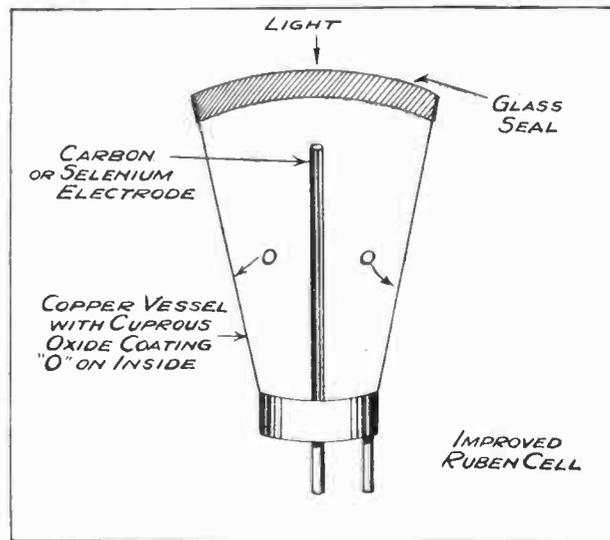
Fig. 4.—Illustrating an improved Ruben Cell.
