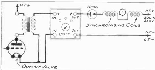
*Fig. 6.—Showing how simple are the connections for a transformer and choke combination.*
