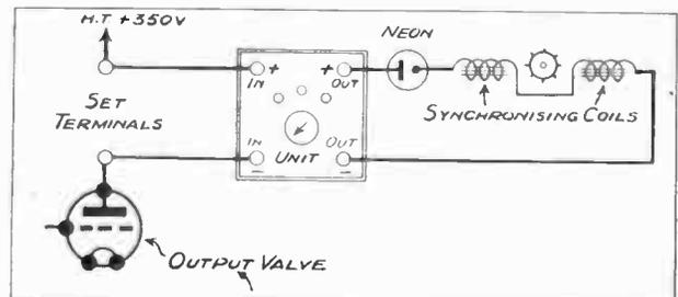
Fig. 5.—With a transformer output in the vision wireless receiver the unit is joined up in this manner.
