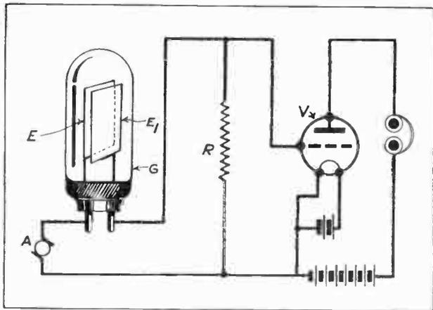
Fig. 3.—A cuprous oxide cell, Ruben's condenser type, together with the requisite electrical circuit.
