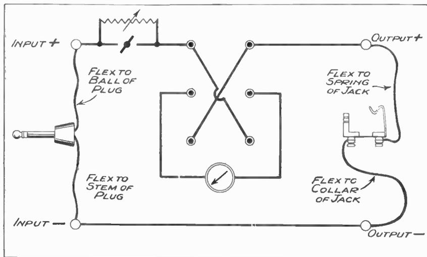
Fig. 2.—The theoretical diagram of the "output controller," showing how the switches, jack, etc., are arranged.
