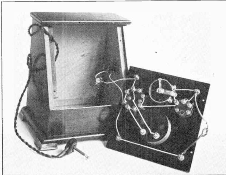
With the panel removed from the small cabinet we can see how the leads are joined to the jack.
