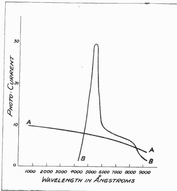
Fig. 2.—A shows an ordinary frequency current characteristic, while B is taken with equal spectral energies.
