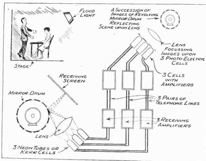
*Pictorially representing the three-zone television scheme demonstrated by the Baird Co.*
