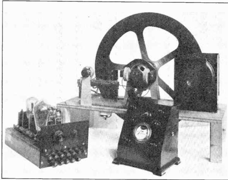
The unit ready for connecting between the vision amplifier and "Televisor" made up from a Baird set of parts.
