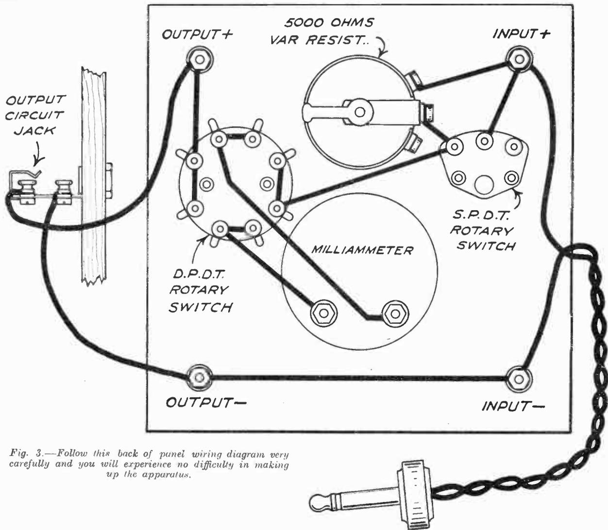
Fig. 3.—Follow this back of panel wiring diagram very carefully and you will experience no difficulty in making up the apparatus.
